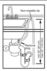
Note: Plumbing installations will vary - refer to local codes. Drain hose included is 79" (201 cm) and can be extended to a maximum of 155 3/4" (396 cm).
