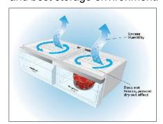
Pores in the VitaFresh™ membrane are bigger than a water vapor molecule, so humidity can easily evaporate through. This provides unmatched food preservation.
