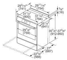
measurements in inches and (mm)
