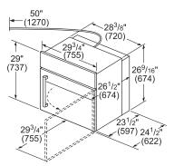
Allow 3/4" (19 mm) gap to nearest cabinet face for door swing on SideOpening models
