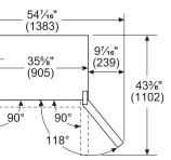
Drawers can be pulled out with door open to 90°. Drawers can be taken out with door
