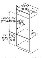
\* Junction box may be installed above, below or to the left or right of the unit within range of the power conduit
