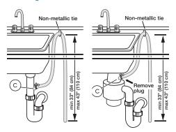
Note: Plumbing installations will vary - refer to local codes. Drain hose included is 90 1/2" (230 cm) and can be extended to a maximum of 168 1/2" (428 cm). Always use the approved drain hose extension kit (SGZ1010UC).
