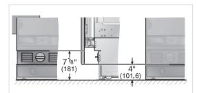
If required by the surrounding cabinetry design, the distance between the bottom edge of the door panel and the floor can be increased from approx. 4" (102 mm) up to 7  $\frac{1}{8}$ " (181 mm), but should not be decreased. Note, however, that the venting grille and (if applicable) water filter cavity will be visible, even if the door is closed.
