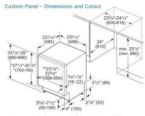
\* measured from the bottom edge of the countertop panel thickness recommended 3/4" (20 mm). This dishwasher can accept custom door panel weights ranging from 7 to 24 lbs: however, the dishwasher comes from the factory ready for custom panel door weights from 11 to 18 lbs. If you plan on using a door panel that is not 11 to 18 lbs.
