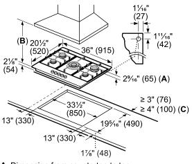
A: Dimension from countertop to top of grates in front of 2<sup>%</sup>/<sub>16</sub>" (65) B: When installed in combination with a hood, refer to hood manufacturer's requirements for installation C: For installation in a kitchen island
