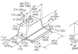
Installation height above cooking surface: 24"-34" (610-864) to Electric 29<sup>1</sup>/2"-34" (750-864) to Gas measurements in inches (mm)
