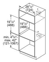
\* Receptacle may be located above or beneath the unit within reach of the power cable.
