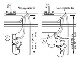
Note: Plumbing installations will vary - refer to local codes. Drain hose included is 90 <sup>1</sup>/2" (230 cm) and can be extended to a maximum of 168 1/2" (428 cm) Always use the approved drain hose extension kit (SGZ1010UC).
