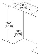
Leave 1/2" (12.7) gap at the top and 1" (25.4) behind the refrigerator for proper ventilation. It is recommended that you do not install the refrigerator near a heat source such as an oven or a range.
