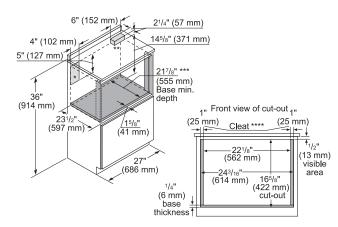
\* Recommended location of electrical outlet \*\* Anti-tip block
