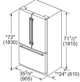
\*Add <sup>5</sup>/8" (17) with front levelling feet fully extended \*\*Add 1" (25) for fixed spacers on back
