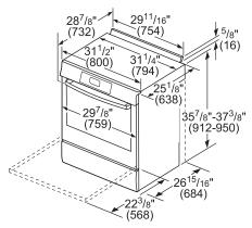
measurements in inches and (mm)
