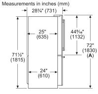
\*Add <sup>5</sup>/8" (17) with front levelling feet fully extended \*\*Add 1" (25) for fixed spacers on back measurements in inches (mm)
