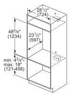
\* Junction box may be installed above, below, or to the left or right of the unit within reach of the power cable
