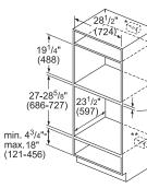
\*Junction box may be located above or next to the unit within the reach of the power cord. \*Junction box may be located below (depending on space) or next to the unit within the reach of the power cord. \*Most combinations available as combo over (one cut out, one electrical hook up)
