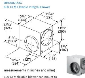
downdraft or be used as an inline blower, and can be rotated to exhaust downward or to sides
