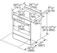
measurements in inches and (mm)
