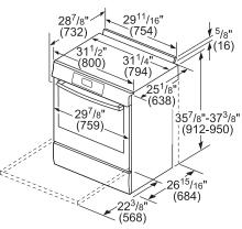
measurements in inches and (mm)
