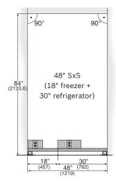
IMPORTANT: Just as with stand-alone columns, always ensure that the receptacles and the water line are correctly positioned. For dimensional requirements see page 211.
