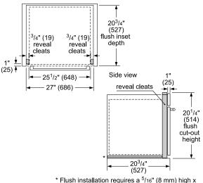
25<sup>1</sup>/2" (648 mm) wide x 19<sup>3</sup>/4" (500 mm) deep base plate underneath the unit body.
