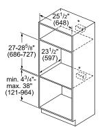
\* For single ovens installed into a wall cabinet, the junction box may be located above or beneath the unit within reach of the power conduit.
