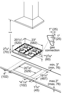
\* 5<sup>1</sup>/16" required when installed with a built-in oven. Reference the Bosch under cooktop built-in guide for more details.
