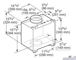
measurements in inches and mm
