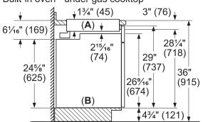
Dimensions based on standard countertop height (36" with  $4\frac{3}{4}$ " toe kick including base plate). A: Cooktop B: Built-in oven
