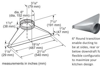
below downdraft for flexible configurations
