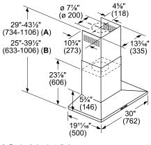
A: Recirculating installation B: Ducted installation
