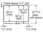
\*The 1<sup>1</sup>/<sub>3</sub>" (34) fixed spacer on back of appliance allows proper ventilation and space for the water connection. measurements in inches (mm)
