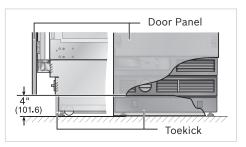
Typical 4" (102 mm) toekick height. Velcro adhesive strips are used to fasten the toekick to the appliance. Venting grille and (if applicable) the water filter cavity are located above the toekick area.
