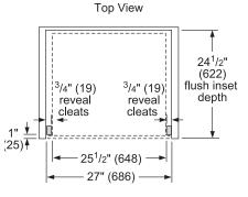
NOTE: See pages 73–81 for planning and installation details when installing Bosch storage and warming drawers in combination with other Bosch products. Horizontal installation of a 27" oven next to a 27" speed oven with warming drawer is possible, but the speed oven and warming drawer require either two cutouts or one cutout with a shelf support in between.
