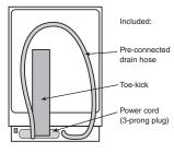
Ensure a portion of the drain hose is raised between min. 33" (84 cm) and max. 43" (110 cm) above the cabinet floor
