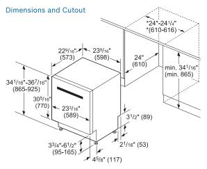
\*23<sup>5</sup>/<sup>8</sup>" (600) without decor strips measurements in inches (mm)
