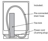
Note: Plumbing installations will vary - refer to local codes. Drain hose included is 79" (201 cm) and can be extended to a maximum of 155 3/4" (396 cm).
