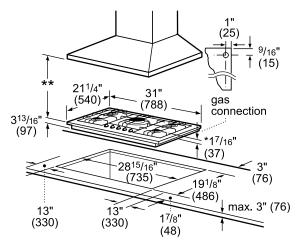
\* Dimension from countertop to top of grates in front of  $1^{7}/16^{"}$  (37). \*\* When installed in combination with a hood, refer to hood manufacturers requirements for installation.
