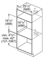
\* Receptacle may be located above or beneath the unit within reach of the power cable.
