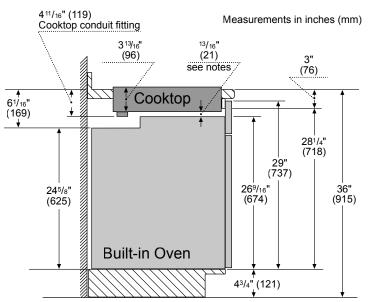
Dimensions based on standard countertop height (36" with 4<sup>3</sup>/<sub>4</sub>" toe kick including base plate).
