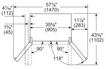
Drawers can be pulled out with door open to 90°. Drawers can be taken out with door completely opened.
