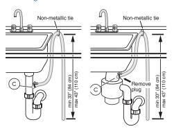
Note: Plumbing installations will vary - refer to local codes. Drain hose included is 79" (201 cm) and can be extended to a maximum of 155 3/4" (396 cm).
