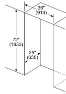
Leave  $\frac{1}{2}$ " (12.7) gap at the top and 1" (25.4) behind the refrigerator for proper ventilation. It is recommended that you do not install the refrigerator near a heat source such as an oven or a range.
