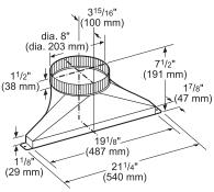
NOTE: HDDSTRAN8 side / rear / downward transition required for side, rear or downward exhaust applications with inline and remote blowers.
