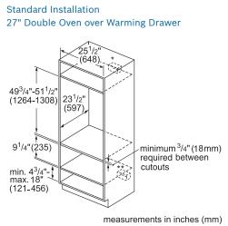
\*Wall oven junction box may be located above or right or left of the unit within reach of the power conduit.
