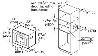
Bean and water reservoir are removed to the front. Recommended installation height 37<sup>1</sup>/2"-57" (95-145 cm).
