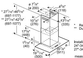
Installation height above cooking surface: 24"-34" (610 mm-864 mm) to Electric 27"-34" (686 mm-864 mm) to Gas.
