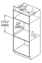
\* Receptacle may be located above or beneath the unit within reach of the power cord.
