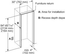
A: Area for installation of power connection. B: Recess depth depends on kitchen design.
