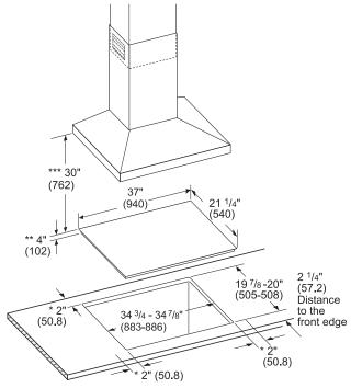
\* Minimum distance from the cooktop cutout to the wall \*\* Maximum cutout depth \*\*\* Minimum distance between the cooktop surface and lower edge of the exhaust hood. Dimensions in inches (mm)
