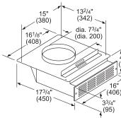
When ducting to the exterior is not feasible, downdraft recirculation kit allows filtered air
