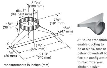
enable ducting to be at sides, rear or below downdraft for flexible configurations
