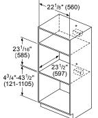
\* For wall installations, the junction box may be located above or below the unit within reach of the power conduit.
