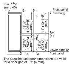
A: Air outlet  $\ge 31^{"2} (\ge 200 \text{ cm}^2)$ B: Ventilation space in the base  $\ge 31^{"2} (\ge 200 \text{ cm}^2)$
