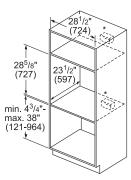
For installation into a wall cabinet, the receptacle may be installed above, below, or to the left or right of the unit within range of the power cord.
