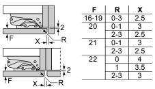
The gap dimensions recommended in the table must be maintained to guarantee collision-free opening of appliance doors and avoid damage to kitchen furniture.
