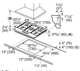
A: Dimension from countertop to top of grates in front of  $2^{23}$ /<sub>64</sub>" (60) B: When installed in combination with a hood, refer to hood manufacturer's requirements for installation C: For installation in a kitchen island
