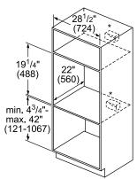
\* Receptacle may be located above or beneath the unit within reach of the power cord.
