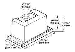
Installation height above cooking surface: 24"-34" (610-864) to Electric 291/2"-34" (750-864) to Gas. measurements in inches (mm)
