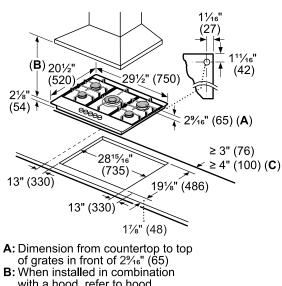
with a hood, refer to hood manufacturer's requirements for installation **C:** For installation in a kitchen island
