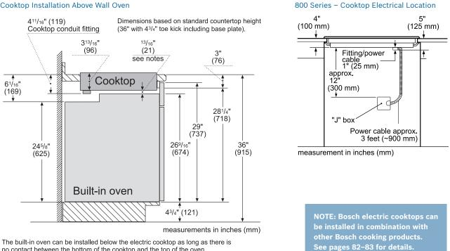
The built-in oven can be installed below the electric cooktop as long as there is no contact between the bottom of the cooktop and the top of the oven.
