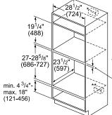
\*Junction box may be located above or next to the unit within reach of the power cord. Junction box may be located below (depending on space) or next to the
