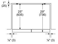
Drawers can be pulled out with door open to 90°. Drawers can be taken out with door completely opened.
