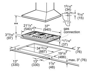
Dimension from countertop to top of \* grates in front of  $1^{7}/16^{"}$  (37). \*\* When installed in combination with a hood, refer to hood manufacturers
