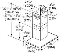
\* Recirculating installation \*\* Ducted installation
