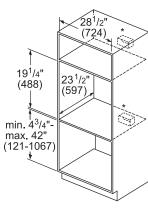
\* Receptacle may be located above or beneath the unit within reach of the power cord.
