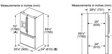
A: Add <sup>5</sup>/<sub>8</sub>" (17) with front leveling feet fully extended B: Add 1" (25) for fixed spacers on back
