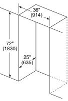
Leave 1/2" (12.7) gap at the top and 1" (25.4) behind the refrigerator for proper ventilation.
