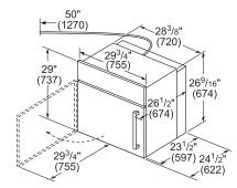
Allow 3/4" (19 mm) gap to nearest cabinet face for door swing on SideOpening models
