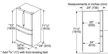
fully extended \*\* Add 1" (25) for fixed spacers on back measurements in inches (mm)
