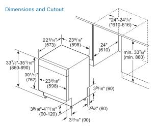
\*235/8" (600) without decor strips measurements in inches (mm)
