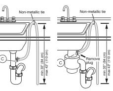
Note: Plumbing installations will vary - refer to local codes. Drain hose included is 75" (190 cm) and can be extended to a maximum of 151" (383 cm)
