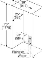
Leave a 1/2" (12.7 mm) gap at the top and 2" (51 mm) behind the refrigerator for proper ventilation. For installation next to a wall, leave a minimum gap of 3<sup>3</sup>/4" (95.2 mm) on the wall side for
