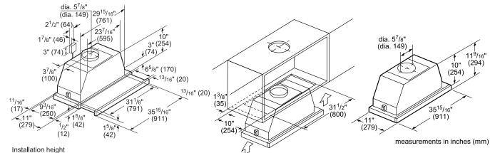
above cooking surface: 24"-34" (610-864) to Electric 291/2"-34" (750-864) to Gas measurements in inches (mm)
